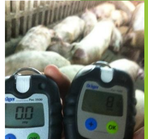
Test Stable NH 3 & H 2 S monitoring
